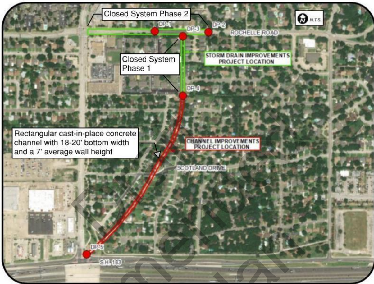
Figure F.61. Channel improvement on Brockbank Channel Basin north of SH 183 (FMP 0330000101)
