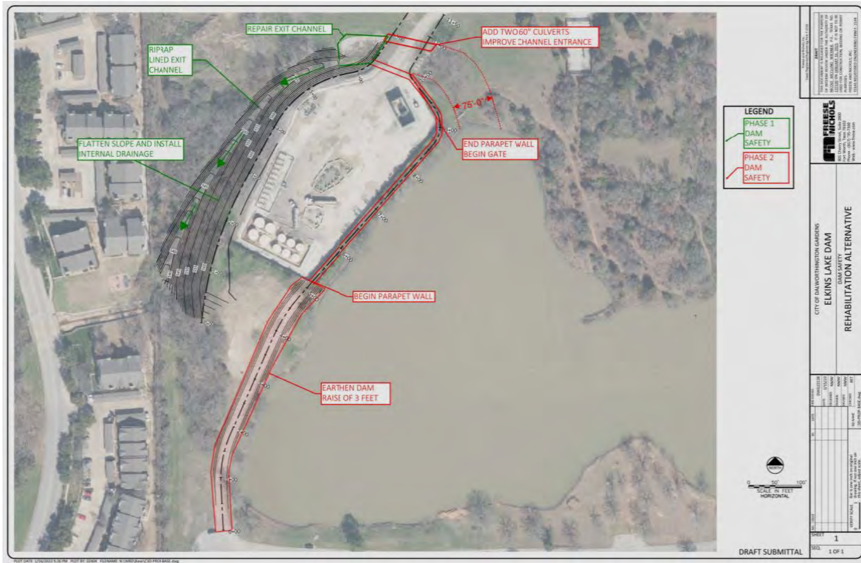
Figure F.31. Elkins Lake Dam Rehabilitation (FMP 033000072)
