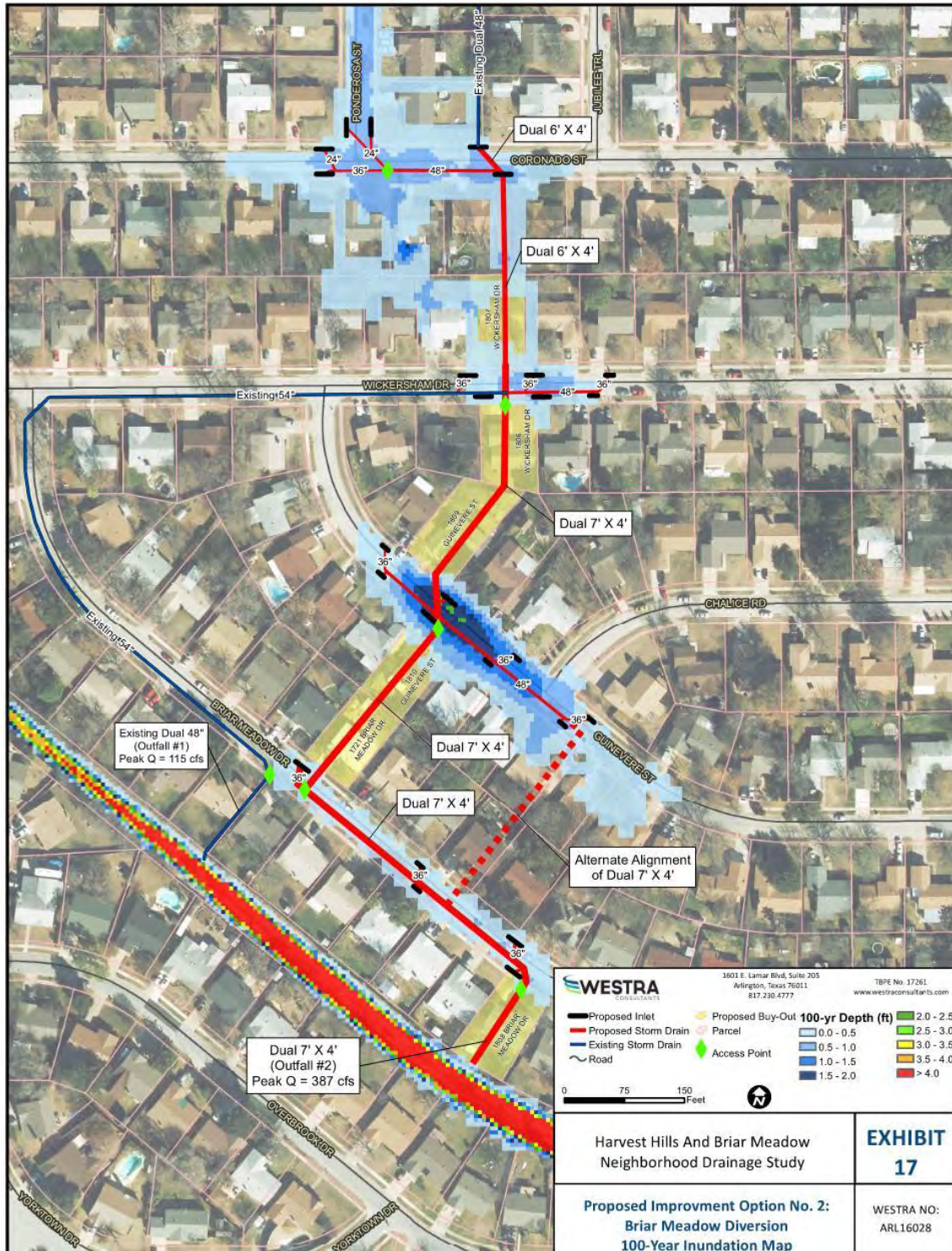
Figure F.45. Arlington Harvest Hills Channel and Drainage Improvements (FMP 033000085)
