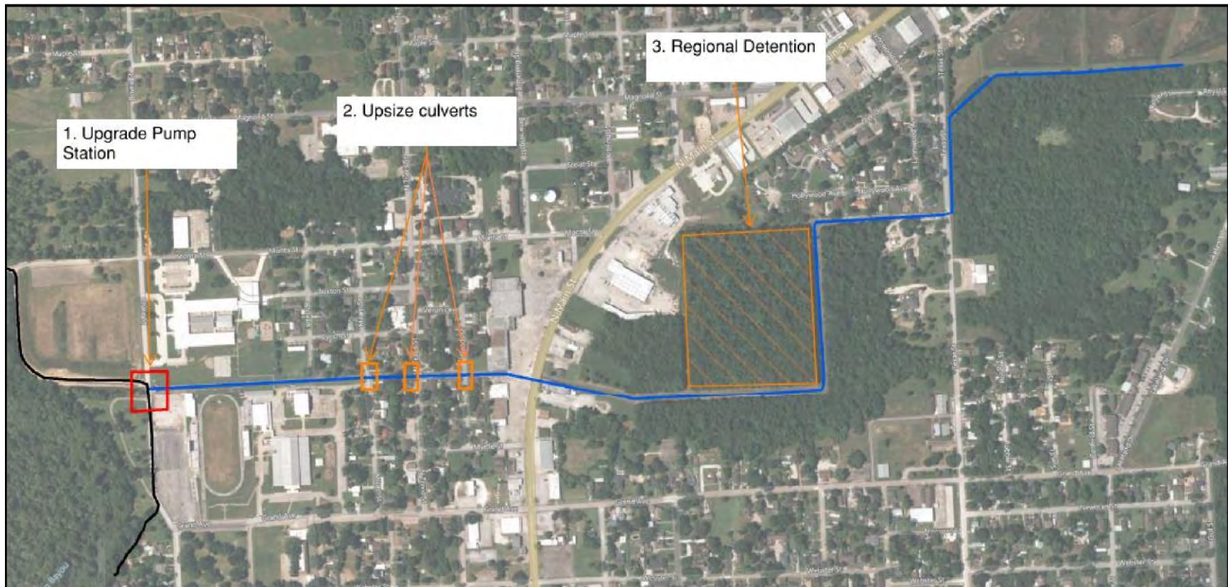
Figure F.38. Main B pump station, detention, and conveyance improvements (FMP 033000078)
